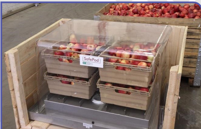
A SafePod unit monitors stress and remaining storage life of apples in a commercial store. Image: Storage Control Systems Ltd
