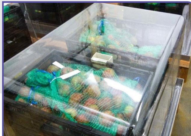
LabPod units (a variant of SafePod) being used to run trials on the stress responses of apples to different storage conditions.
